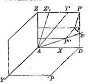
to the new axis of Z', and through Q, the point in which the parallel pierces the plane X'Y', draw QP'' parallel to the axis Y'. Then will AP''=x', QP''=y', P'Q=z', be the co-ordinates of the point (P, P'), referred to the new system of co-ordinate planes.
